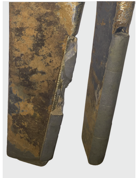
Photos after 200 hectares on a 4 meter machine. Adaptable tine on the left / KUHN tine on the right.
