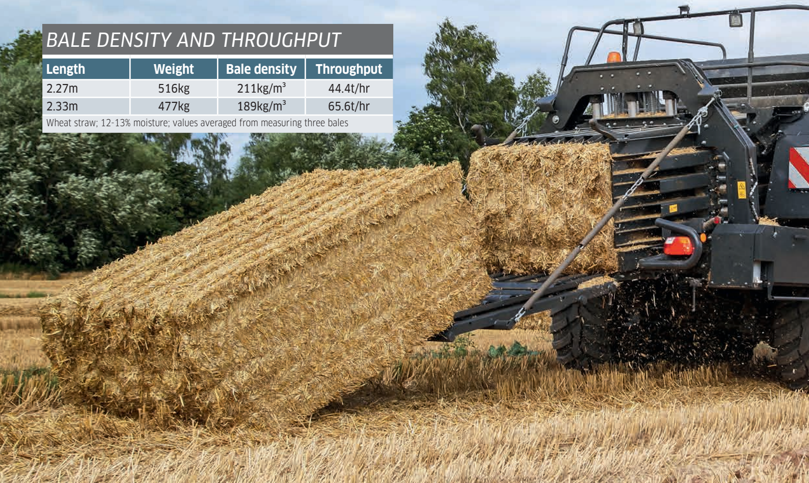
The six double knotters produce short offcuts, but powerful fans keep the area clean.
