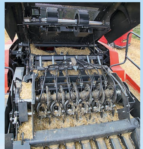
The six double knotters produce short offcuts, but powerful fans keep the area clean.
