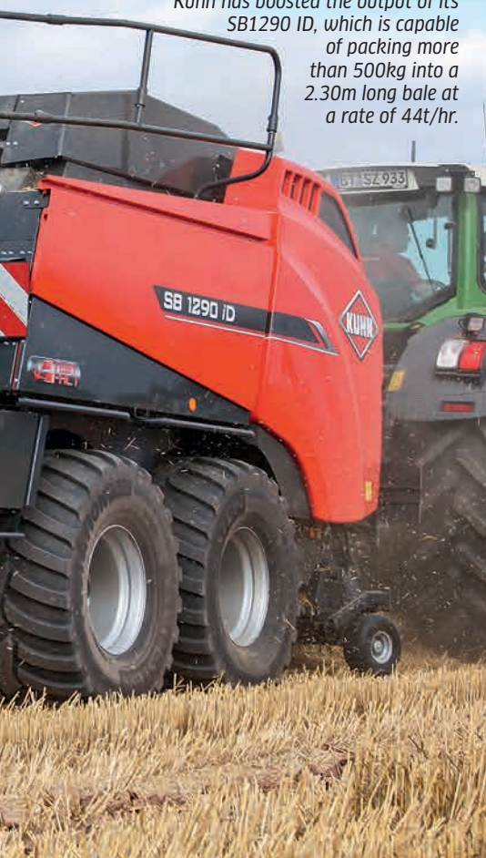
The pick-up is now 13cm wider and boasts a powered 250mm diameter feed roller ahead of the rotor. The roller 'adapts' to swath shape.
