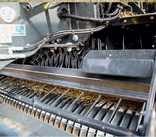
The pick-up is now 13cm wider and boasts a powered 250mm diameter feed roller ahead of the rotor. The roller 'adapts' to swath shape.
